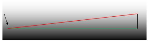
In simple terms, the static rake angle is adjusted in the garage by changing the static ride height settings. If you set the front ride height to 20mm, and the rear to 40mm, then the rake angle is steeper than if you have the ride heights set at 20mm-and-30mm front-to-rear.
